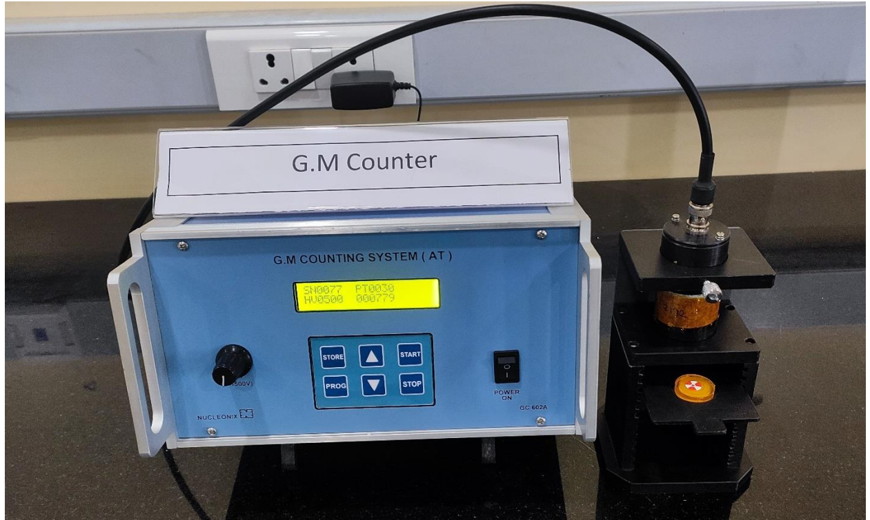
Experiment Setup for Characteristic of GM Tube (Figure 1.1)
