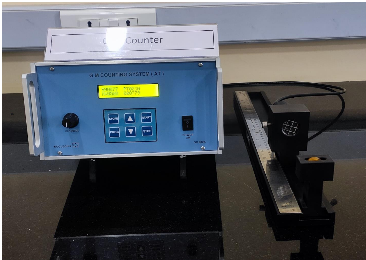
Experiment Setup for Inverse Square Law (Figure 2.1)
