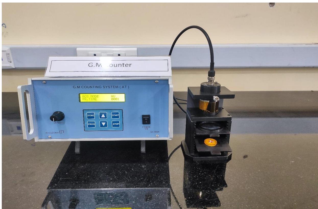
Experimental Setup for Beta particle Range (Figure 3.1)
