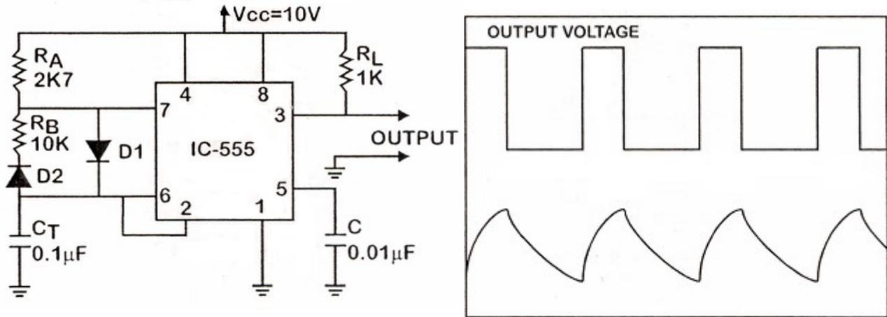
**Astable multivibrator with duty cycle variable from 0 to 100%:**
