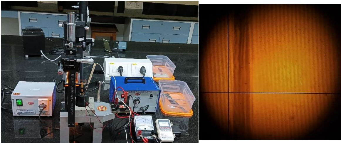
Fig. 4: Experimental set up and the Fizeau's fringes
