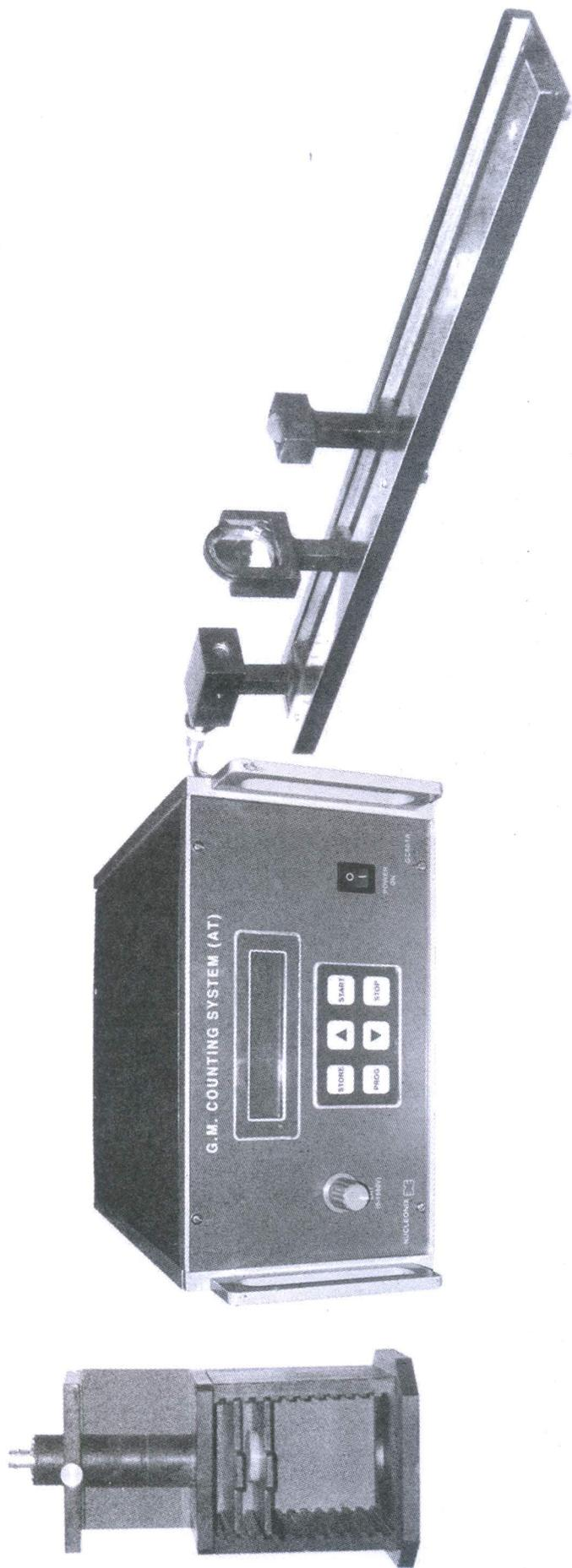
**Fig. 1: G.M. Counting System with G.M. Detector (End Window) stand and
