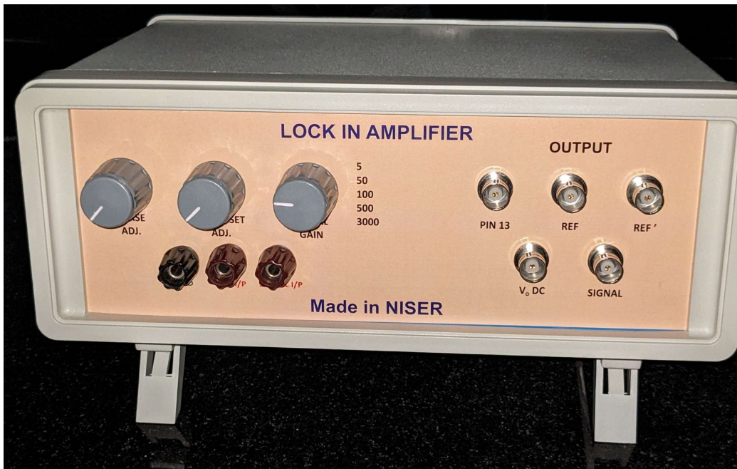
Figure I. Lock-in Amplifier front panel
