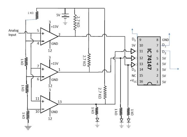
Figure 2. Circuit diagram for 2 bit binary Anolog to Digital conversion
