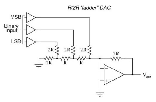
Figure 1. Circuit diagram for digital to anolog conversion
