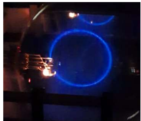
Fig. 4(b): Circular trajectory of electron beam observed in dark
